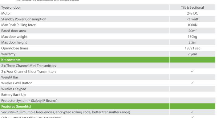
Sub 1 watt in standby (use less energy) DC motor (soft start/soft stop, quiet)
