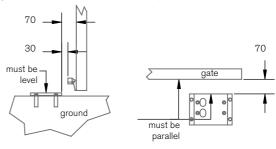
exactly parallel to the gate. The edge of the plate should be 40 mm from the face of the gate.
